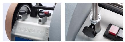
On the new T-8 model, Tormek has integrated the previous mounted sleeves for the Universal Support into the fully cast housing. That guarantees minimal play for the Universal Support; an innovation which improves the control of the sharpening and increases the accuracy of the final results.
