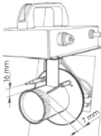
Check the distance of the electrode and the safety thermostat.
